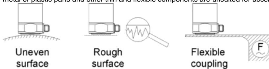
Figure 15: Typical reasons of coupling errors
