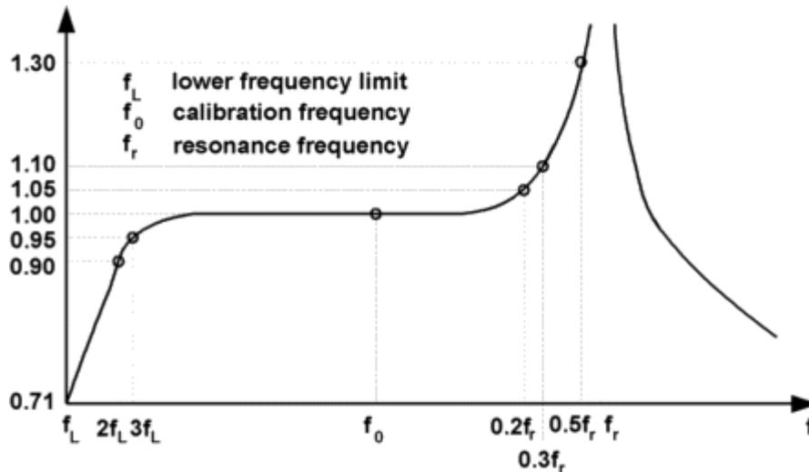
Figure 3: Typical frequency response of accelerometers
