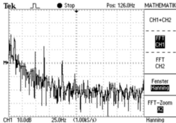
Figure 9: Typical noise spectrum of an IEPE compatible accelerometer
