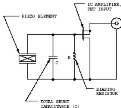
Figure 2: Schematic of LIVM Force Sensor
