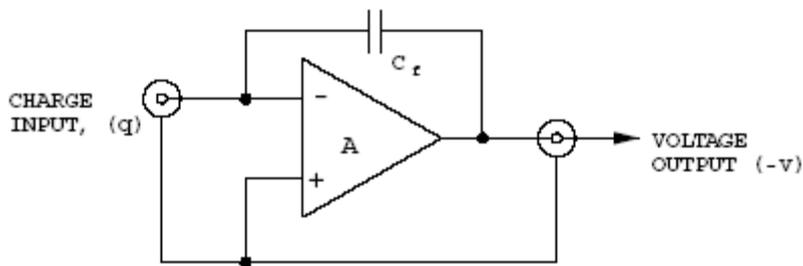
Figure 3: Charge Amplifier, Simplified Schematic
