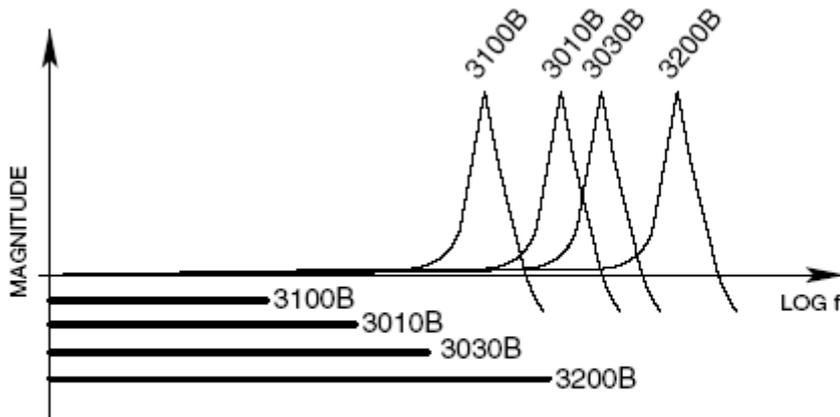
Figure 4: High Frequency Response Comparison
