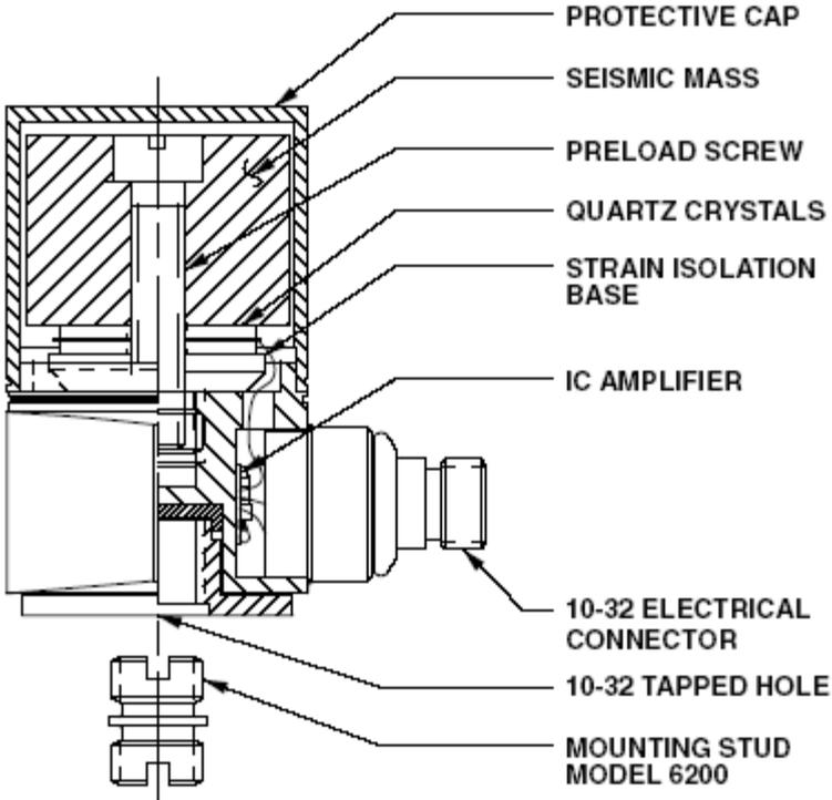
Figure 1: Compression design LIVM accelerometer.
