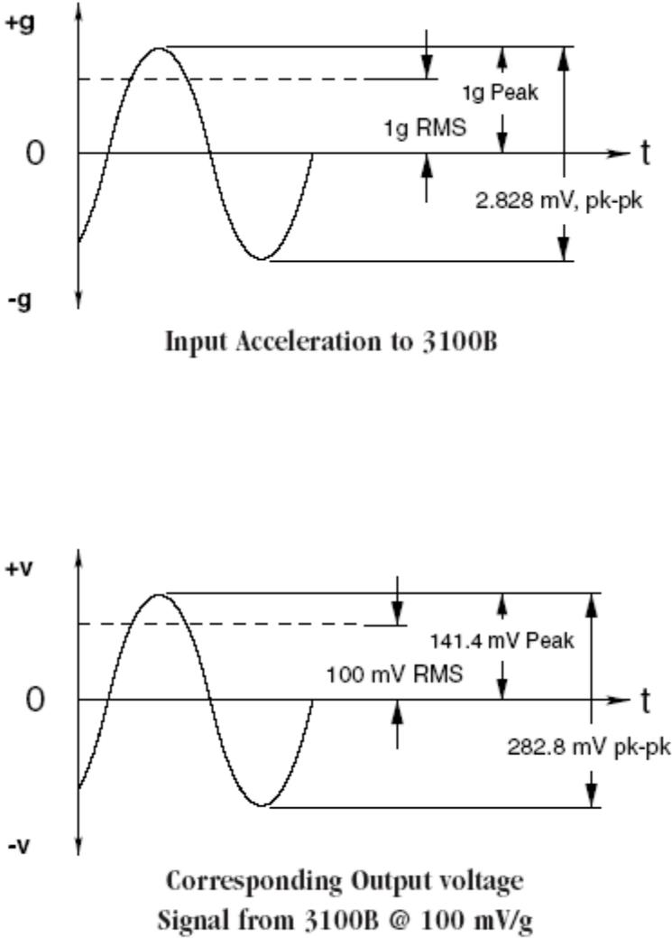
Figure 5: Input/Output Waveforms
