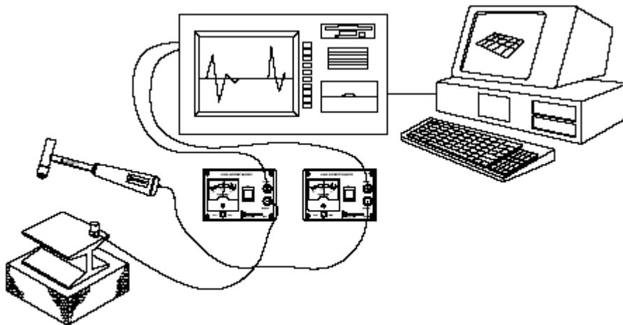
Figure 7: Typical Impulse Hammer Analysis System
