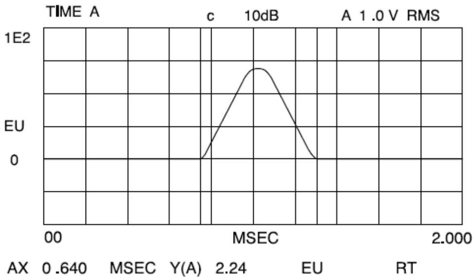
Figure 5: Hammer Pulse, No Extender, Hard Plastic Tip
