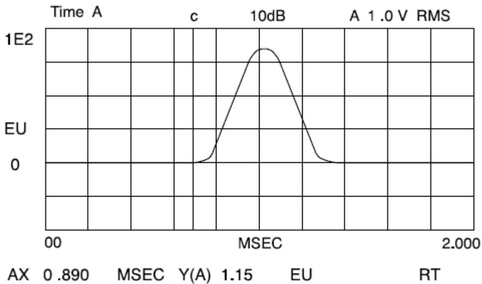
Figure 6: Hammer Pulse, One Extender, Hard Plastic Tip
