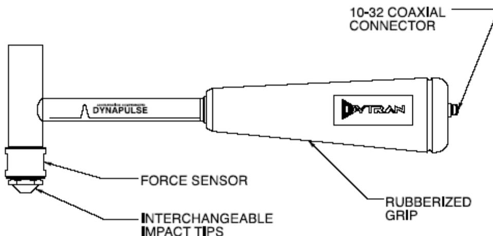
Figure 1: Impulse Hammer Structure
