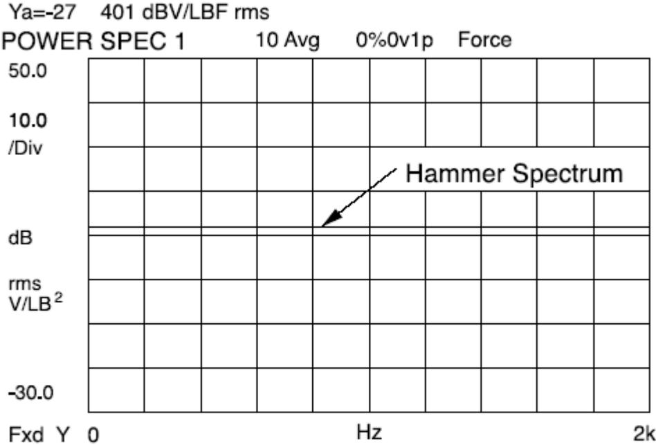
Figure 2: Impulse Spectrum, Aluminum Tip, No Extender
