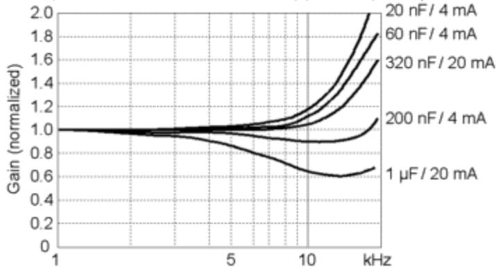
Figure 7: Frequency response of IEPE accelerometers for different cable capacitances and supply currents
