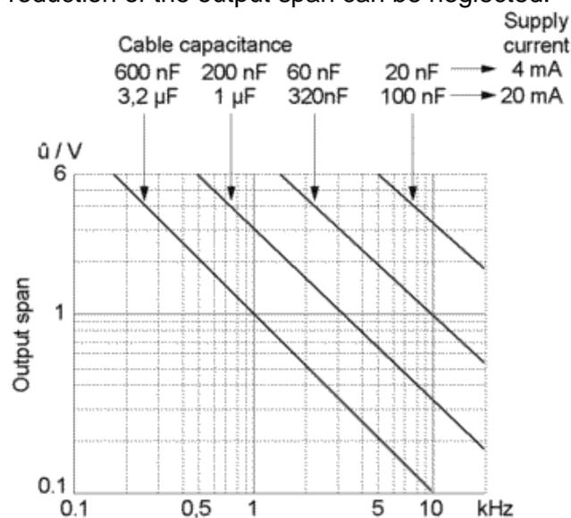
Figure 6: Output span of IEPE accelerometers for different cable capacitances and supply currents
