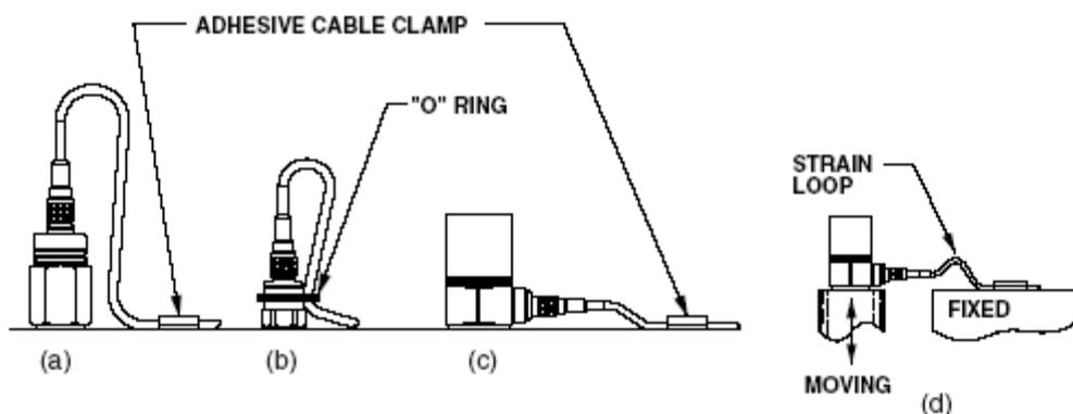
Figure 1: Various Methods of Cable Tie-down
